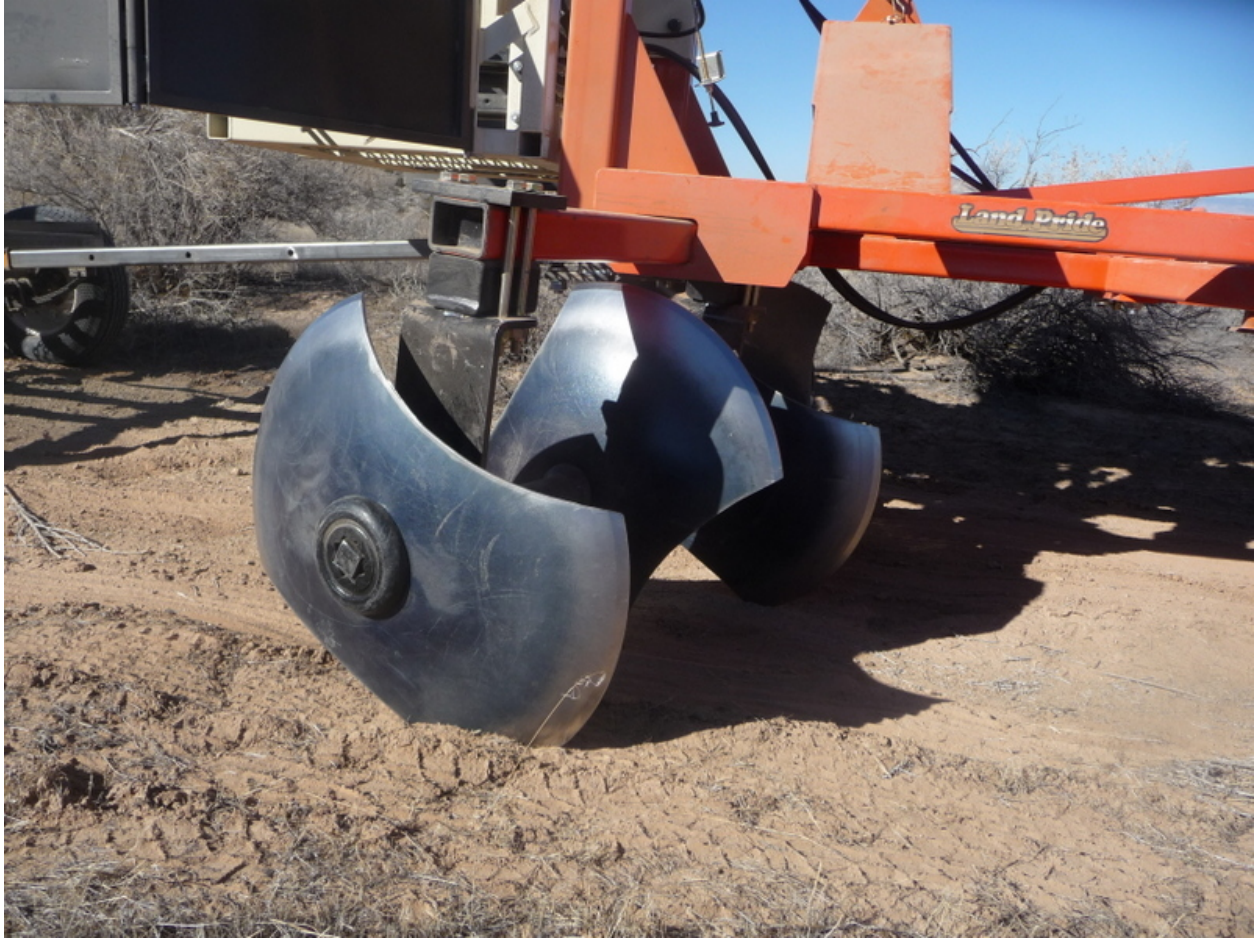
Figure 3. Disks were deeply notched on the pothole seeder, and the notches were offset on adjacent disks.
