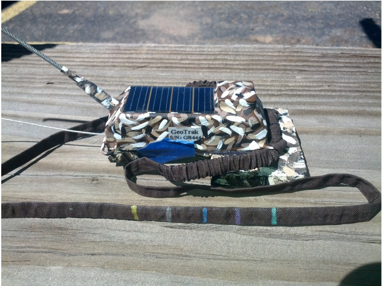
Figure 3. Improved harness and transmitter design for rump-mounted leg-loop attachment of solar-powered GPS satellite PTT transmitters for male greater sage-grouse. This photo also shows the underside placement of a micro-VHF mortality sensor/transmitter.
