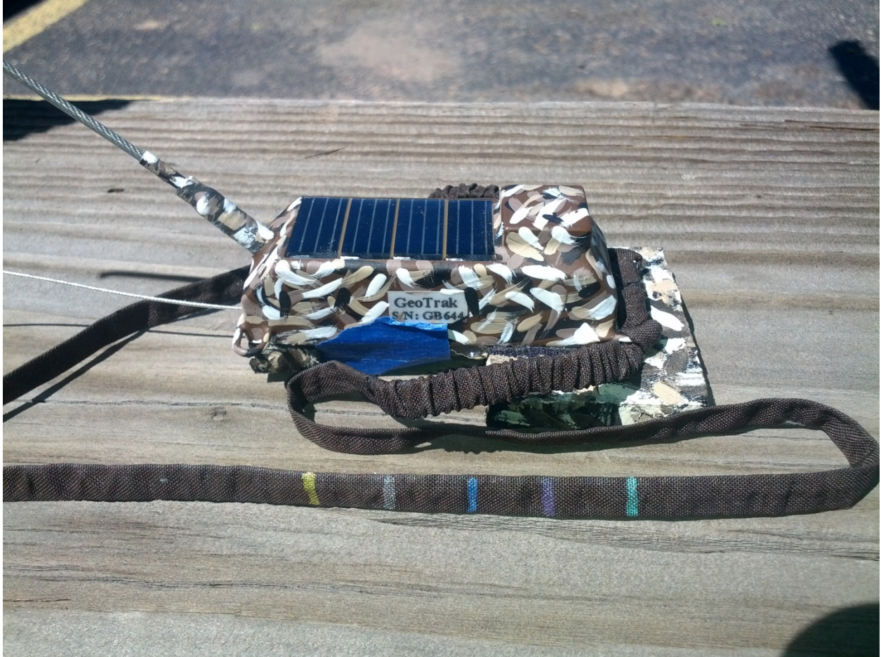
Figure 3. Improved harness and transmitter design for rump-mounted leg-loop attachment of solar-powered GPS satellite PTT transmitters for male greater sage-grouse. This photo also shows the underside placement of a micro-VHF mortality sensor/transmitter (with the magnet held in place with blue painter's tape).
