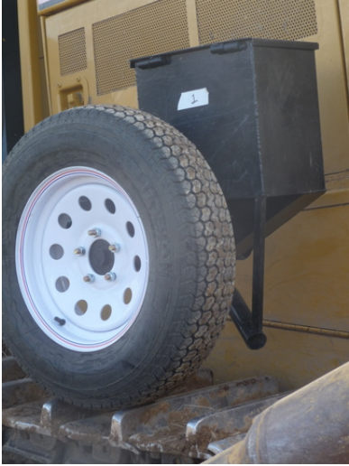
Figure 3. Hansen-style seed dribbler mounted to the track of bulldozer. Two such dribblers were mounted on each bulldozer.
