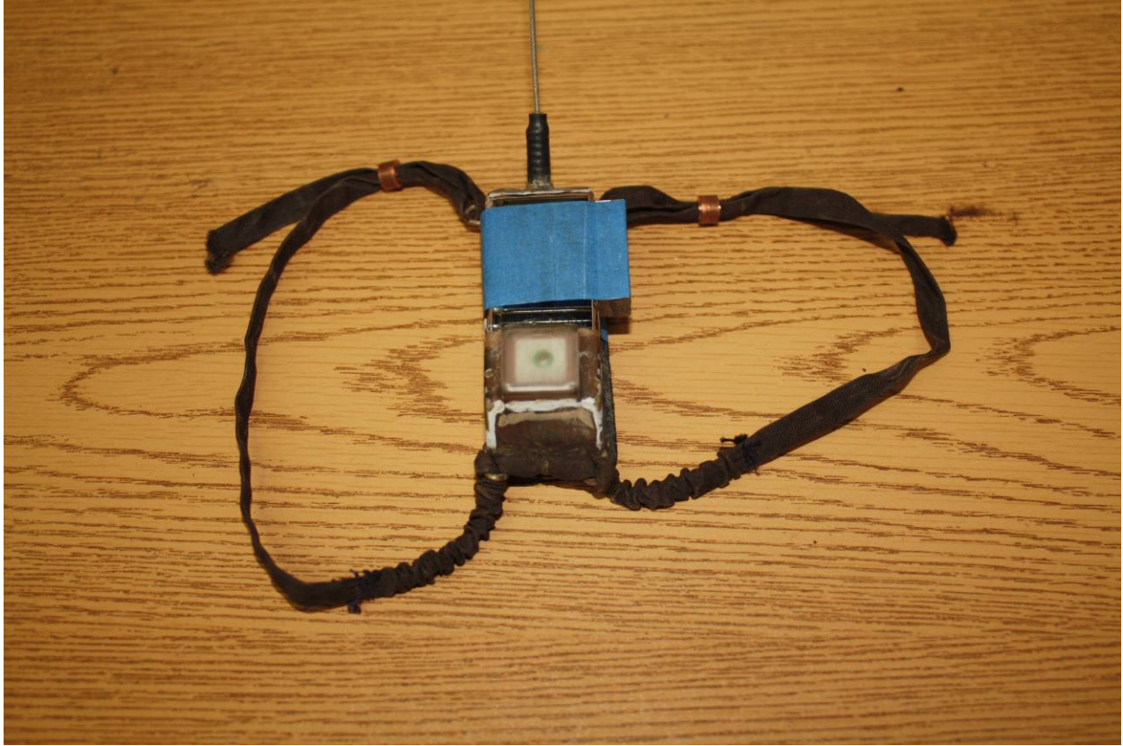
Figure 2. Harness design for rump-mounted leg-loop attachment of solar-powered GPS satellite PTT transmitters to male greater sage-grouse.
