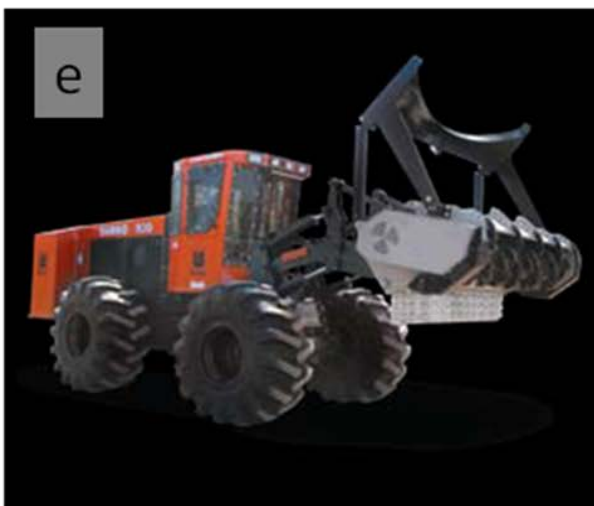
Figure 2. Types of machinery used and woody debris produced: Ship anchor chaining (a) and tree skeletons left behind by chaining (b); roller chopper (c) and coarse debris left by roller-chopping (d); drum-style hydro-axe (e) with fine debris left behind by hydro-axing (f).
