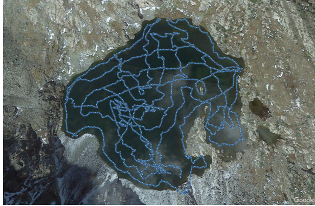
Figure 3: Fifteen depth transects were run on Lower Winchell Lake and projected on Google Earth.
