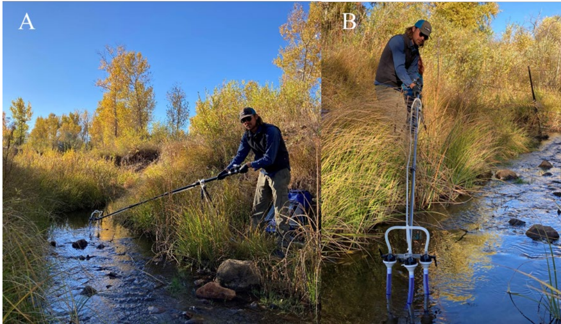
Figure 1. Smith Root eDNA backpack sampler. Note the triplicate collection system. Water is collected and run through filters in the blue backpack seen at the feet of the technician. Photo credit: Boyd Wright.
