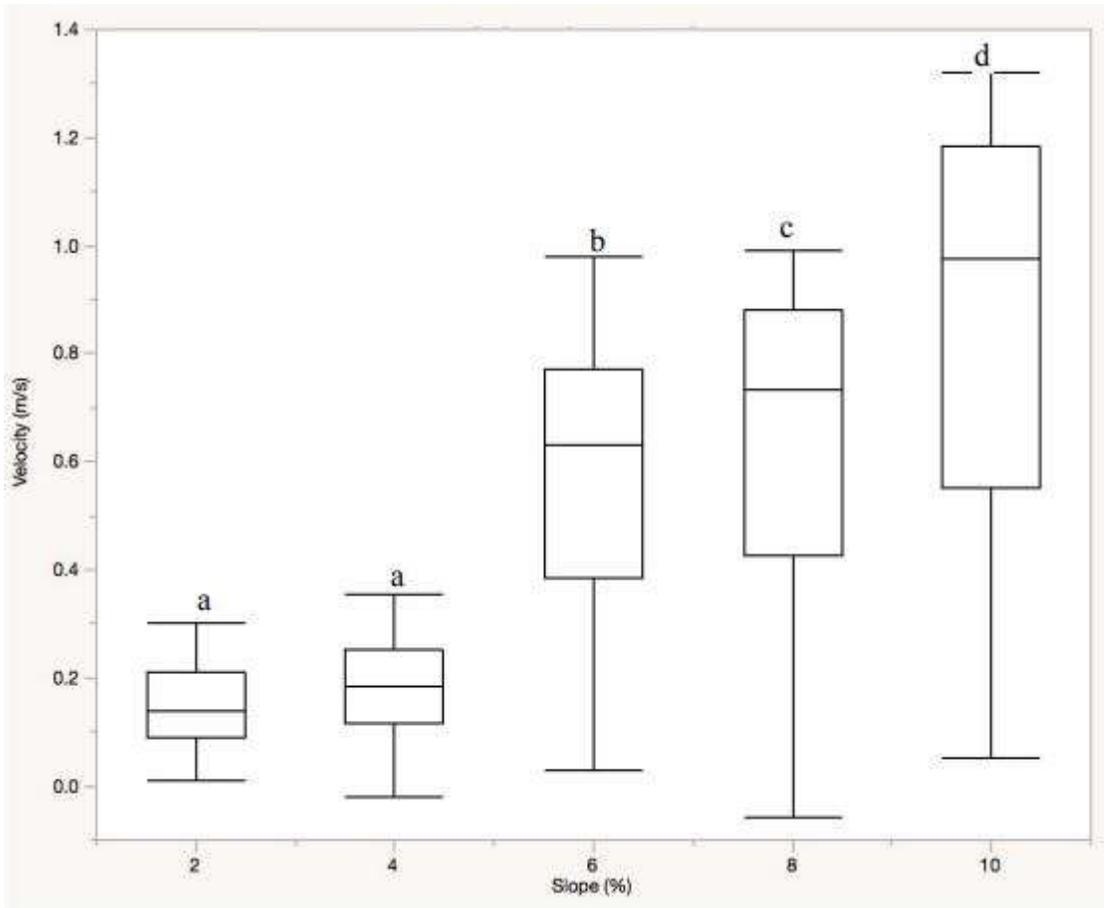
**Figure 7.** Box-and-whisker plots of slope and velocity for the Colorado State University Foothills Fisheries Laboratory rock ramp fishway. Letters indicate statistically significant differences at  $\alpha < 0.05$ .
