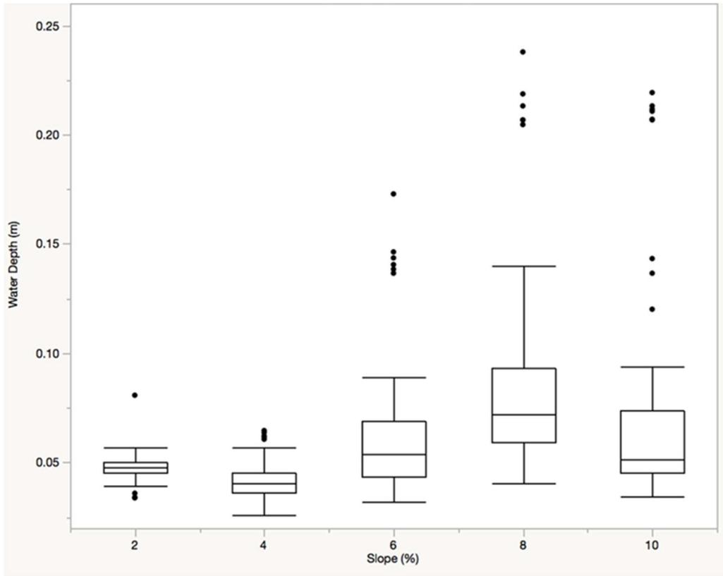
**Figure 5.** Box-and-whisker plots of slope and water surface elevation for the Colorado State University Foothills Fisheries Laboratory rock ramp fishway. Letters indicate statistically significant differences at  $\alpha < 0.05$ .
