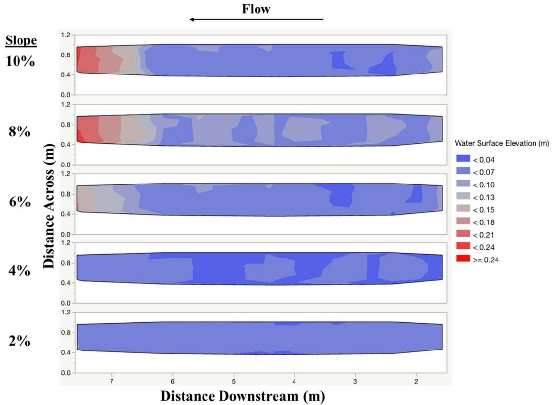
**Figure 4.** Contour plots of water surface elevations throughout the fishway at five slopes. Water surface elevations were taken using a point gauge at 58 points in 19 cross-sections.
