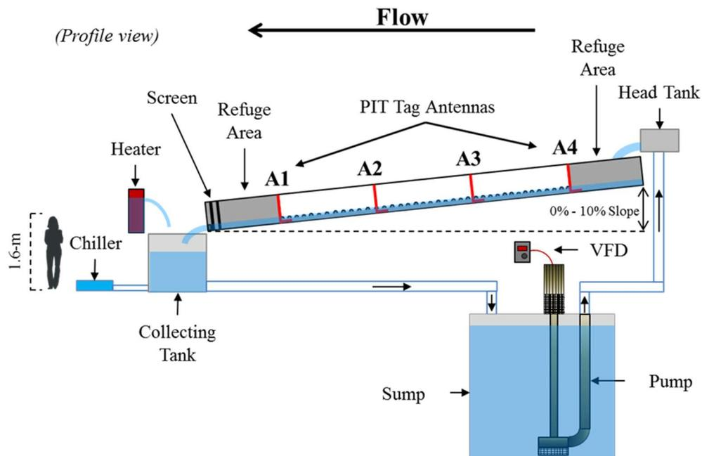
**Figure 1.** Diagram of the research flume built at the CSU Foothills Fisheries Laboratory. The flume is a closed recirculating system equipped with a 4,800-watt heater and large
