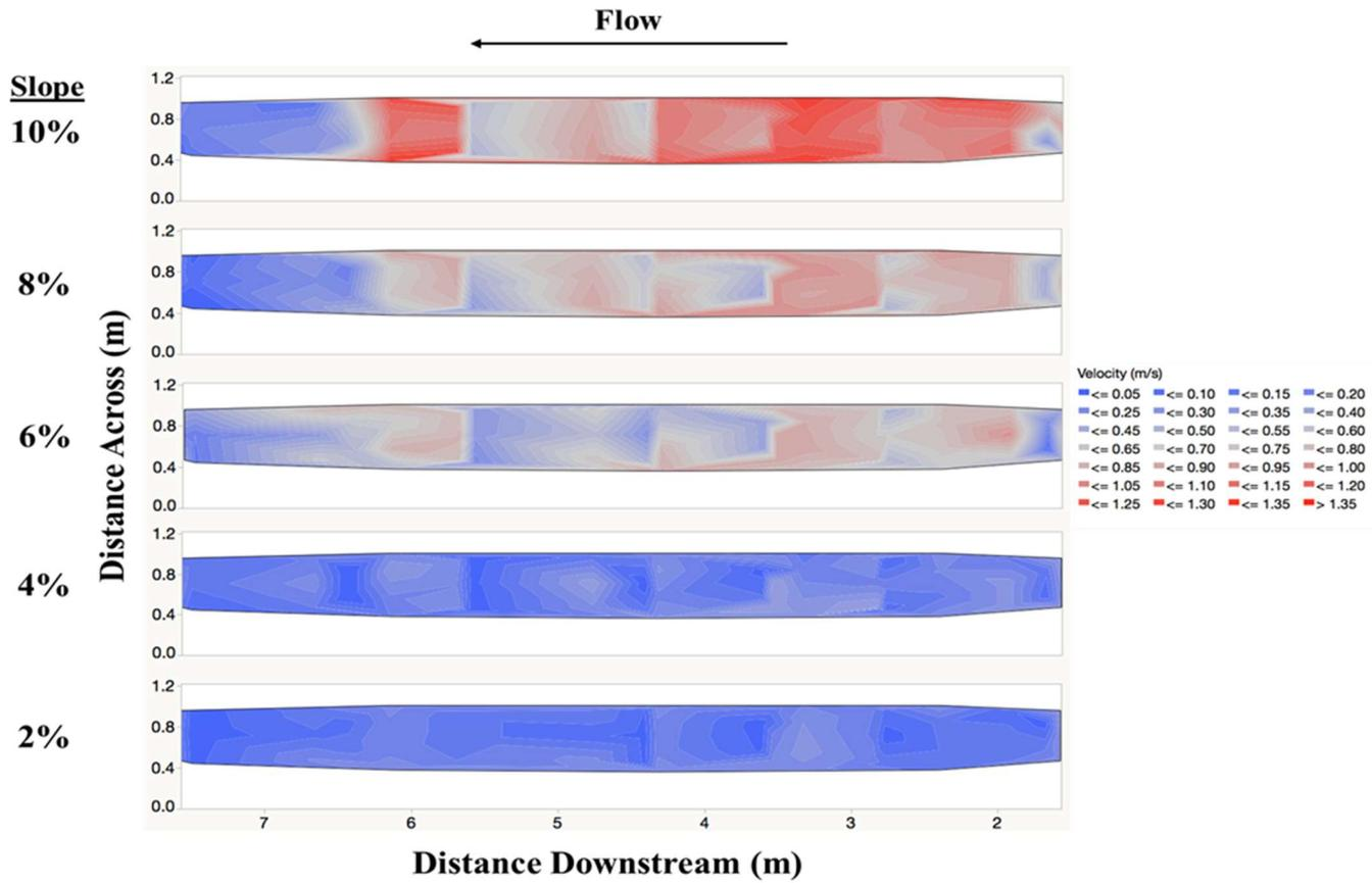
**Figure 6.** Contour plots of the velocity measurements taken throughout the rock ramp fishway at five slopes. Depth-averaged velocity measurements were taken using a Marsh McBirney flowmeter at 58 points in 19 cross-sections.
