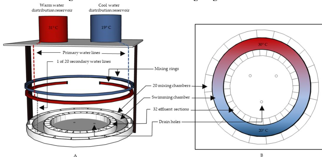
**Figure 7.** Lateral (A) and overhead (B) views of the thermal preference chamber that was used to quantify fish’s thermal preference and movement (modified from Myrick et al. 2004). One of the 20 secondary water lines is shown to provide an
