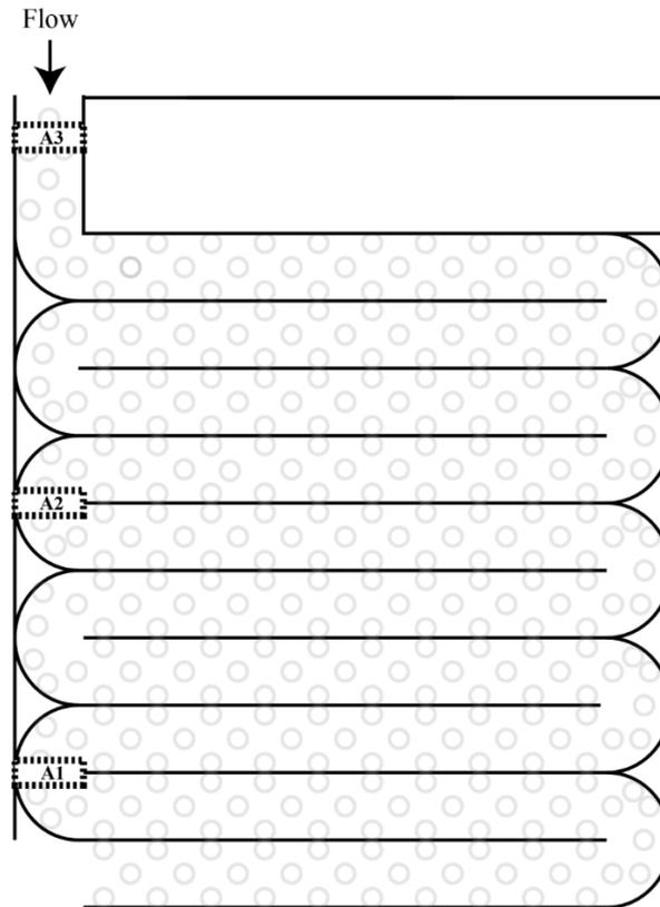
**Figure 3.** Schematic of PIT-tag antenna array within the Longrie-Fecteau fishway at Owens Hall diversion structure. Dashed boxes indicate PIT-tag antennas. Open circles indicate roughness elements. Total travel distance from the entrance of the fishway to its exit = 123.3 m (structure entrance to A1 = 22.3 m, A1 to A2 = 49.7 m, A2 to A3 = 49.7 m, A3 to structure exit = 1.6 m).
