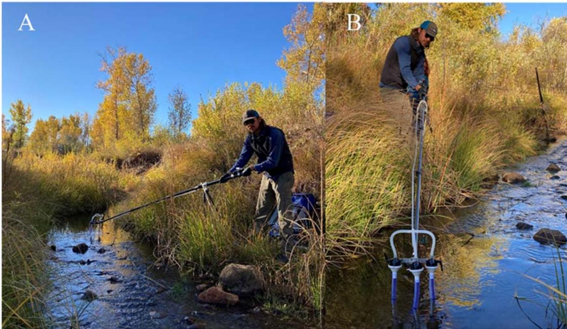
**Figure 6.** ANDe environmental DNA collection system. Note the triplicate collection system. Water is collected and run through filters in the blue backpack seen at the feet of the technician. Photo credit: Boyd Wright.
