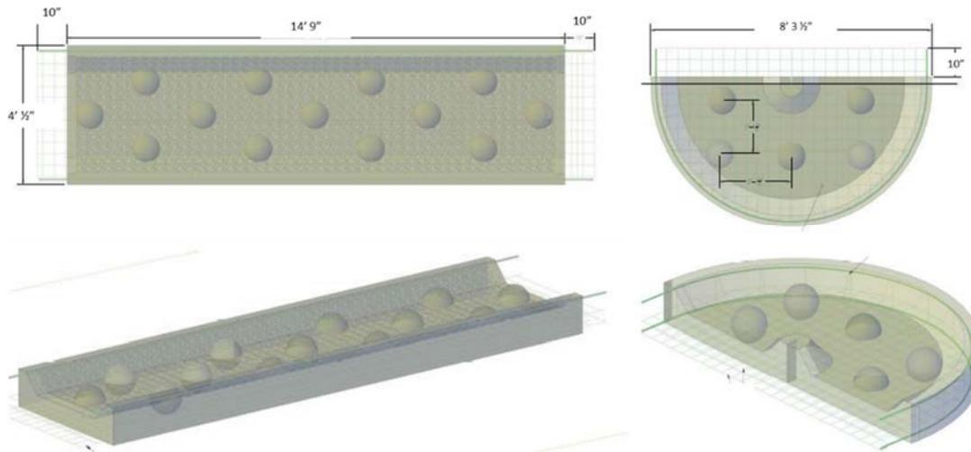
**Figure 2.** Straight and curved sections that make up the Longrie-Fecteau fish passage structure. By adding and removing the number of these prefabricated pieces, the fish passage structure can be adjusted to the height required for a particular barrier.
