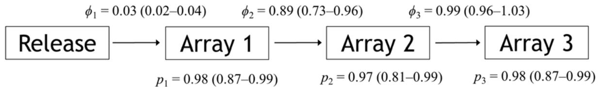
**Figure 4.** Model averaged parameter estimates from a Cormack-Jolly-Seber model to estimate movement ( $\phi$ ) and detection probabilities ( $p$ ) on a conceptual diagram of the Longrie-Fecteau fish passage structure.
