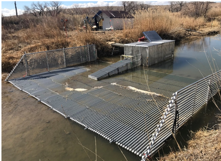
Figure 2. The fully assembled resistance board weir (RBW) in Roubideau Creek. The photo faces upstream. The PVC pickets in foreground are anchored on the upstream end to a substrate rail, but can pivot freely with water level. The only passage through which fish can pass is the PVC chute leading into the aluminum cage. The wall-tent in the back ground houses the fish-working station.
