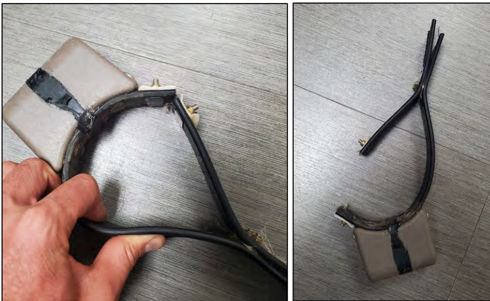
Figure 2: A collar with PCL drop-off placed on study animal NE17 on 6/14/2022. This collar dropped off naturally on 4/6/2024. The PCL spacer broke right down the center line, not near the bolts. This may have been partly due to the bend produced by this shape of collar, sometimes called a “tear-drop” shape. We do not expect to use tear-drop shaped collars for the remainder of the study.
