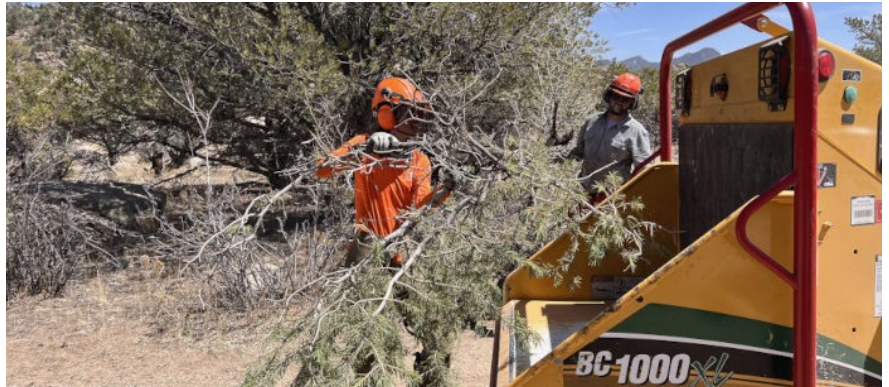
Using a chipper to turn downed trees and thinned branches into mulch is one way to create more defensible space around a home or building. Photo: Mercedes Siegle-Gaither, CSFS
