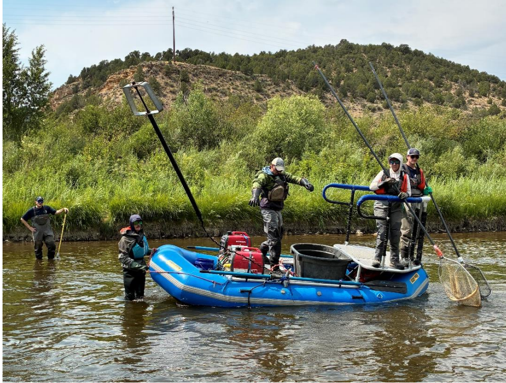
Figure 23. Collecting baseline fish population data using an electrofishing raft with thrown electrode at baseflow conditions of approximately 100 cfs.
