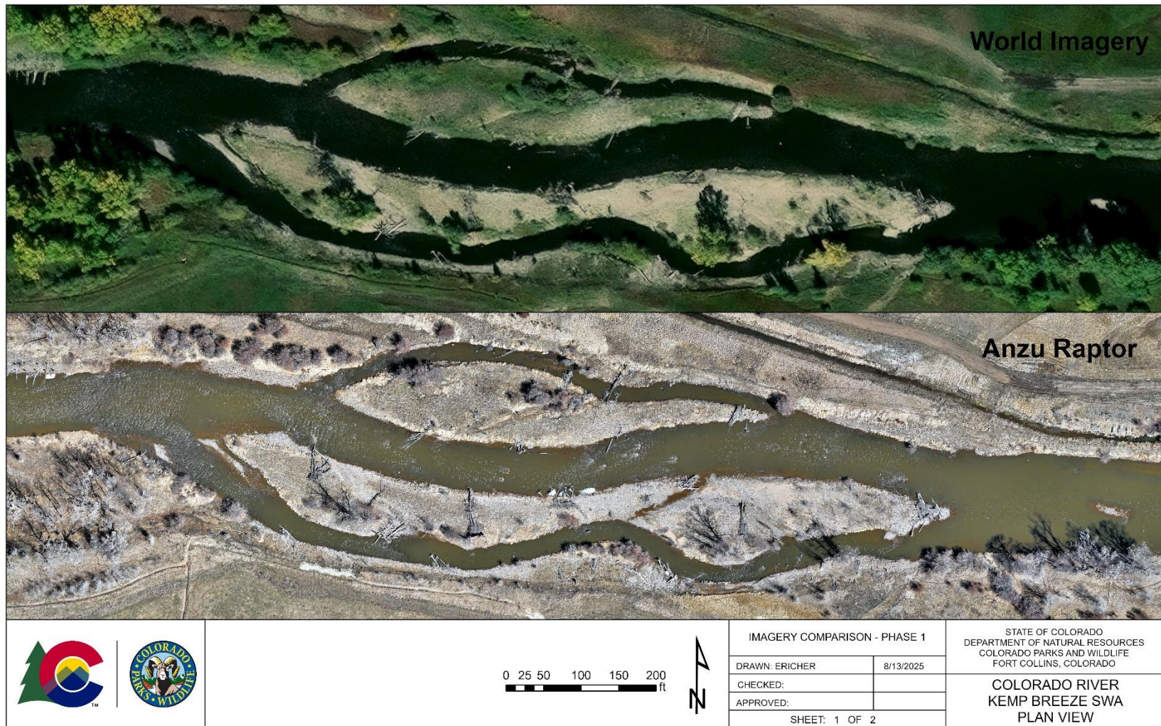
Figure A3. Comparison of standard world imagery basemap (resolution = 0.5 m) and unmanned aerial system (Anzu Raptor) imagery (resolution = 0.02 m) for the Kemp-Breeze SWA Habitat Project, Phase 1 reach.
