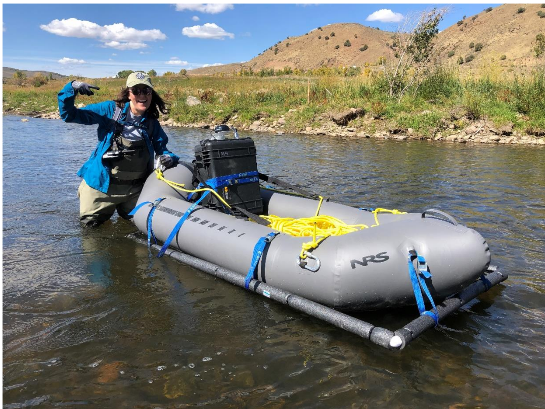
Figure 10. New pack-raft antenna system used to relocate PIT-tagged tracer rocks in 2024.
