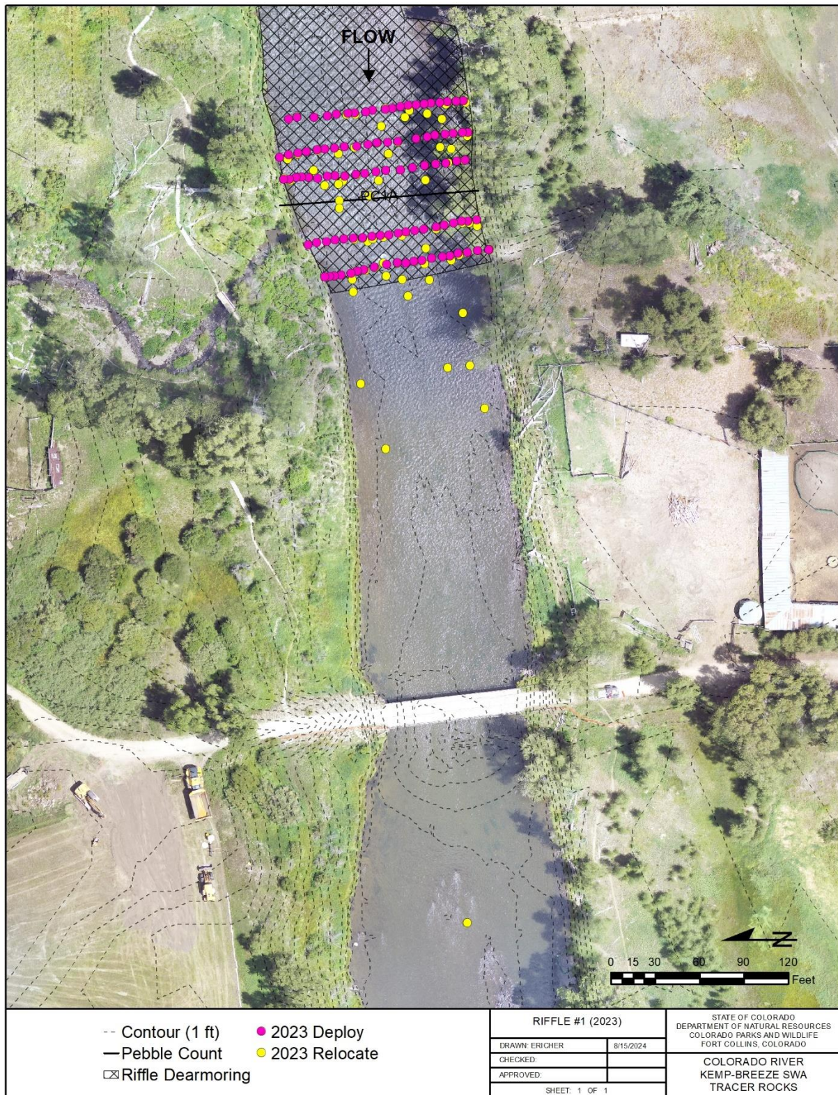
Figure 8. Tracer rock locations following deployment in April 2023 and relocation in October 2023 at an experimental location that was treated with riffle dearmoring (riffle 1).
