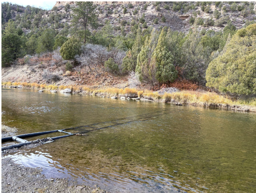
Figure 8. Biomark PIT Tag antenna in the Uncompahgre River at the downstream end of the study section.
