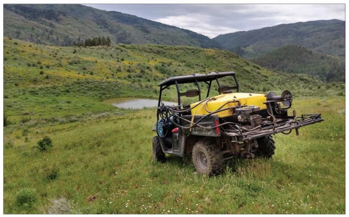
**Figure 3.21.** Utility Terrain Vehicle with herbicide spray tank and hose reel for targeted weed treatments in Route County, Colorado. (Photo: Todd Hagenbuch.)
