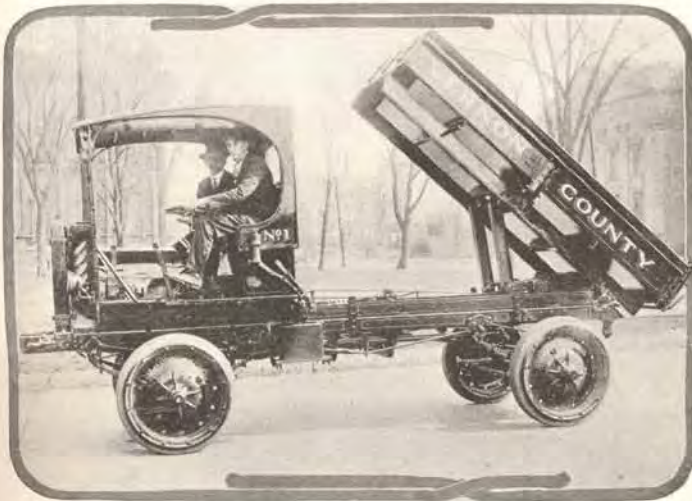
Colorado's new road truck body, of which 100 have been ordered; a "Horizontal Hoist."
