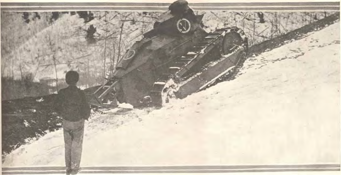
The War Tank making a stiff grade up the motor highway to the summit of Pike's Peak. The Whippet was able to negotiate such drifts without much trouble until the hardening snow broke some of the tractor plates.
