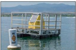
The Standley Lake Profiler is equipped with a multi-probe sonde which provides measurements of water temperature, dissolved oxygen, pH, conductivity, turbidity, oxidation/reduction potential (ORP), fluorescent dissolved organic matter (fDOM), and chlorophyll a concentrations.
