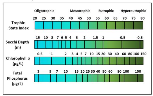
Figure 28. Carlson's Trophic State Index and Corresponding Values for Secchi Depth, Chlorophyll *a*, and Total Phosphorus
