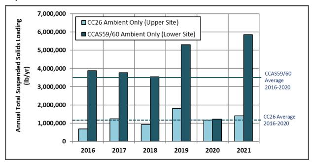
Figure 10. Total Suspended Solids Load Estimates in the Upper Basin, 2016-2021
