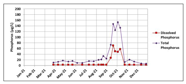
Figure 42. Total and Dissolved Phosphorus Concentrations in Standley Lake, Bottom, 2021
