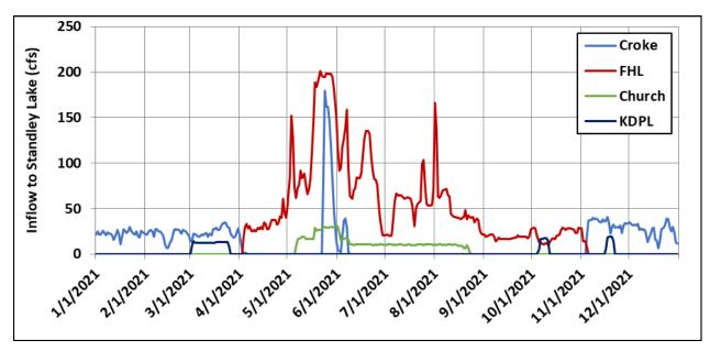
Figure 9. Hydrographs for the four conveyances to Standley Lake, 2021
