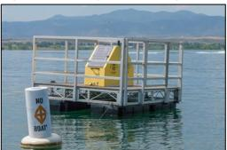
The Standley Lake Profiler is equipped with a multi-probe sonde which provides measurements of water temperature, dissolved oxygen, pH, conductivity, turbidity, oxidation/reduction potential (ORP), and chlorophyll a concentrations.
