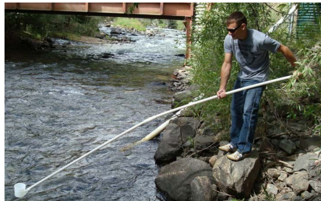
Figure 10. Taking a Grab Sample from Clear Creek at Lawson Gage (CC 26).
