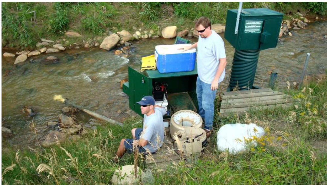
Figure ES-2. Autosampler station on North Fork of Clear Creek (CC AS 50). Gage is the green box on the right, the autosampler is in the middle and the continuous probes/sample collection line is the pipe leading from the creek on the left.
