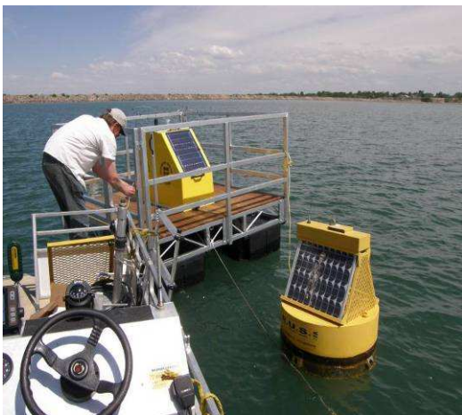
Figure 18. YSI profiler replaces RUSS on Standley Lake.
