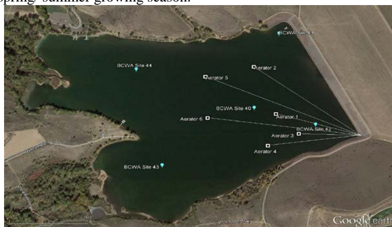
Figure 24 New BCR Aeration Configuration
