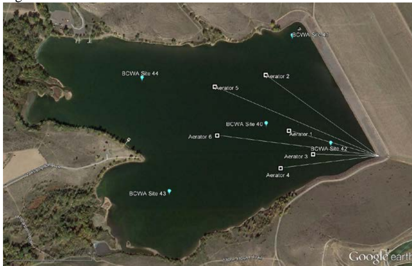
Figure 24 New BCR Aeration Configuration
