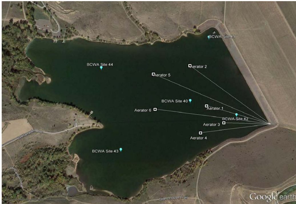
Figure 26 New BCR Aeration Configuration
