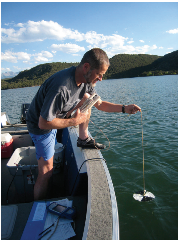
Water Quality Control Division's Jim Saunders measures Secchi depth at a local reservoir.
