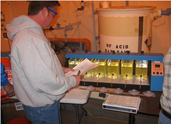
Students in the advanced training sessions brush up on jar testing skills that will help them ensure their plants are operating at their best.
