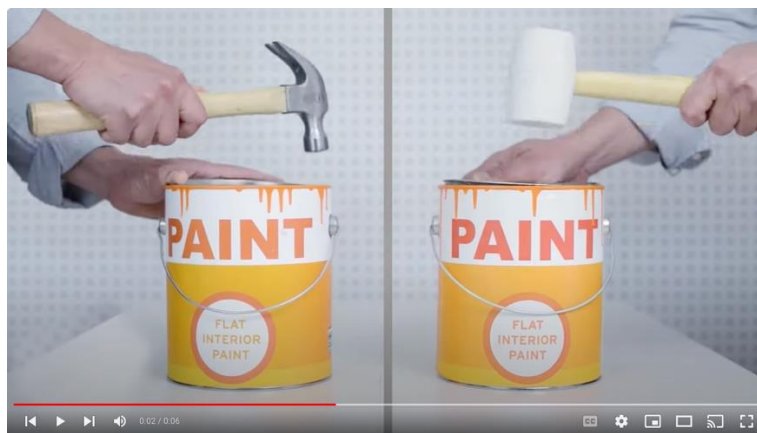
Example of Storage Tip Video Showing Use of a Rubber Mallet to Avoid Damaging Can
