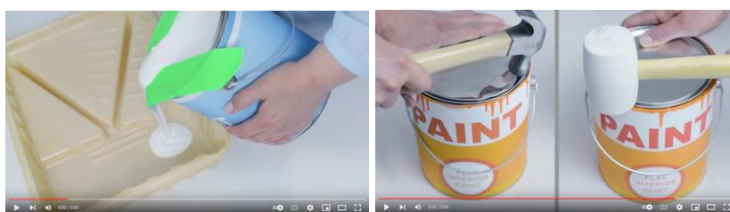
Two Examples of Storage Tip Videos: (1) Create a Tape Spout to Reduce Spills, (2) Use a Mallet to Close a Paint Can (Using a Hammer Can Damage the Can)
