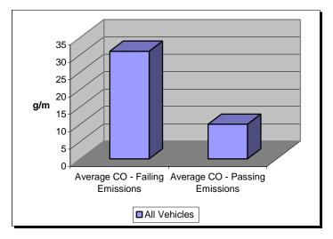
Light-duty trucks that failed their initial test emitted an average of 35 grams of carbon monoxide per mile. On a passing retest these same vehicles emitted an average of 13 grams per mile. This is a 63% reduction in the amount of carbon monoxide emitted by these vehicles. Vehicles that passed the IM240 test on the initial attempt emit an average of 5 grams of carbon monoxide per mile.
