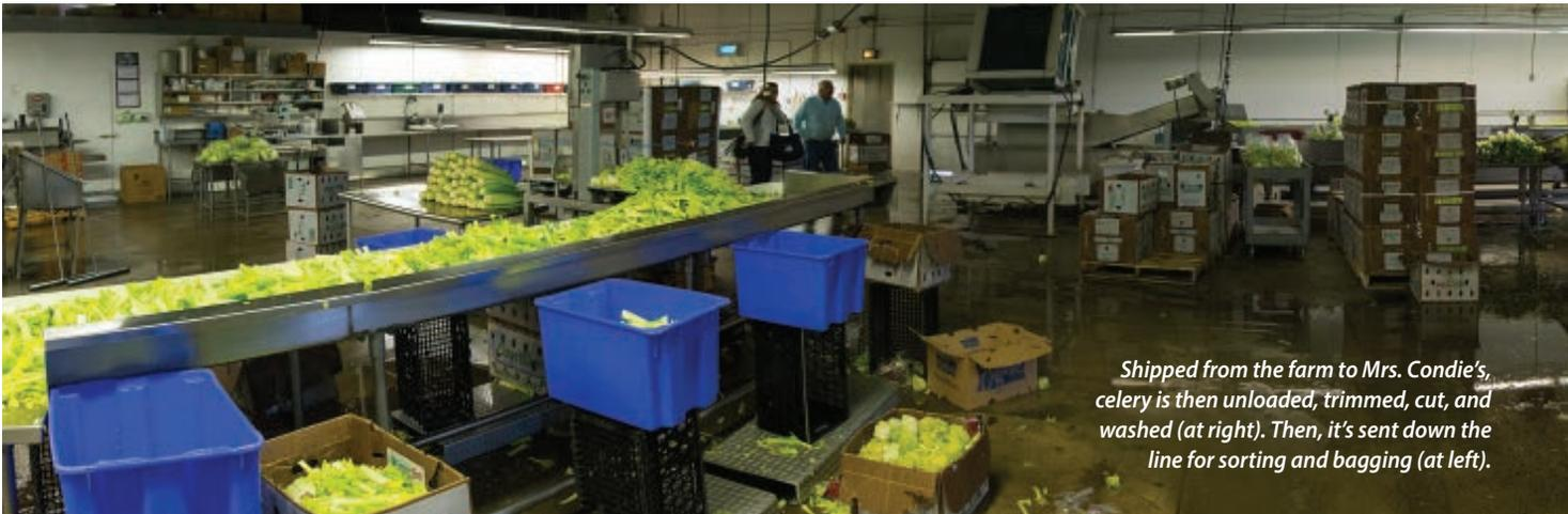
*Shipped from the farm to Mrs. Condie's, celery is then unloaded, trimmed, cut, and washed (at right). Then, it's sent down the line for sorting and bagging (at left).*
