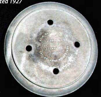
*John Losasso used this “ring packer” to pack fruit and vegetables in bushel baskets without damaging the produce.*
