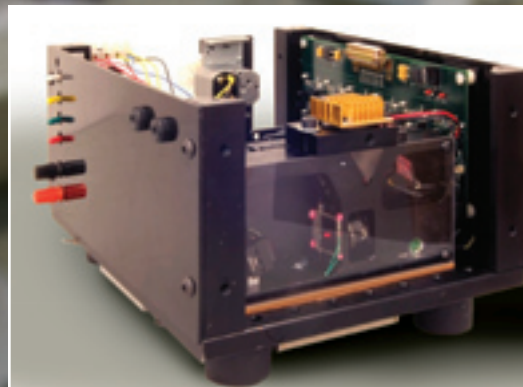
The AlphaSniffer 207B1 can be used to detect very small particles including microRNAs, some of which have been linked to cancer and heart disease. BiOptix President and CEO Misha Plam (pictured at right) says the technology could be used to quickly diagnose heart attacks in hospital emergency rooms. COURTESY BIOPTIX INC.
