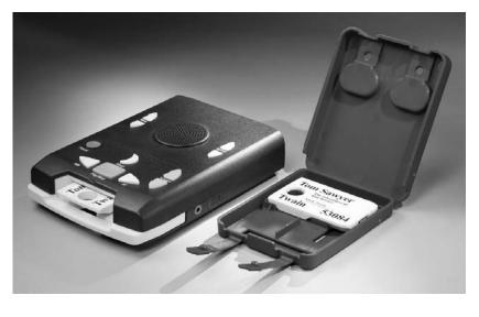
cartridge is about the same size as the current cassette for easy handling. The mailing container is also similar to the current container so the current mailing cards can still be used.
